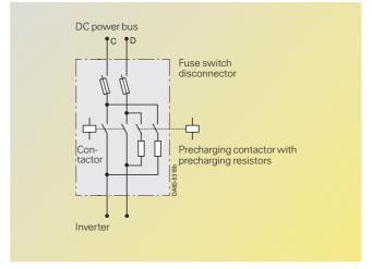
Fig. 6/56 Electrical connection
