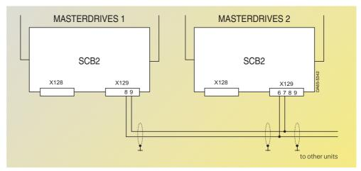
Fig. 6/68 Example of a parallel peer-to-peer connection via RS485
