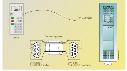
Fig. 6/97 OP1S in a point-to-point link
