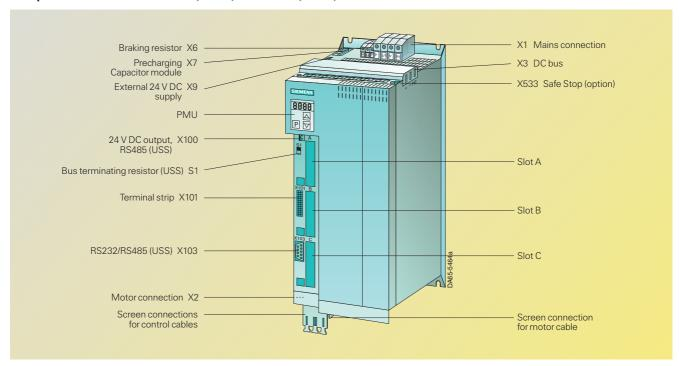
Fig. 6/31 Connection overview for Compact PLUS converters 11 kW (15 HP) and 15 kW (20 HP)
