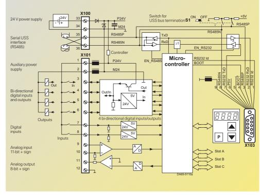
Fig. 6/34 Control terminals of the Compact PLUS inverters
