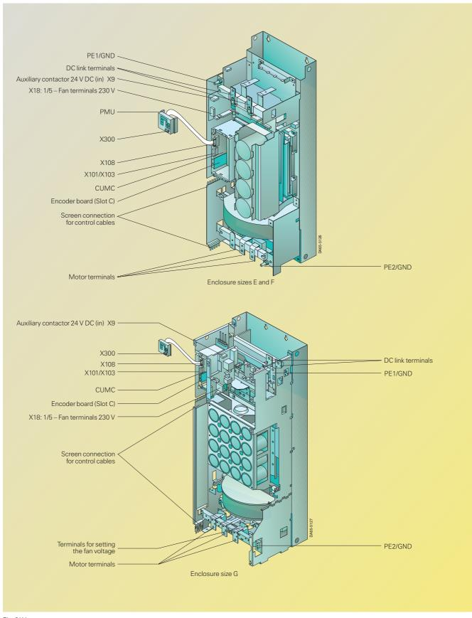
Fig. 6/41 Overview of terminals on the chassis-type inverters
