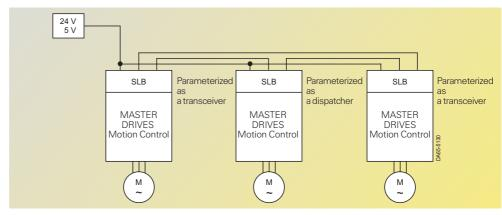
Fig. 6/77 Peer-to-peer functions with SIMOLINK
