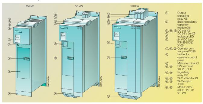
Fig. 6/35 Overview of terminals on the Compact PLUS rectifier units
