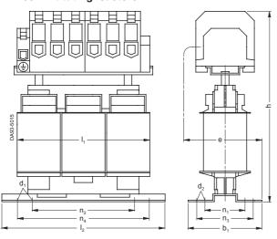
$\ensuremath{\text{n}_{\text{3}}}$  and  $\ensuremath{\text{n}_{\text{4}}}$  mounting hole acc. to EN 60 852-4  $n_1$  and  $n_2$  mounting hole acc. to DIN 41 308
