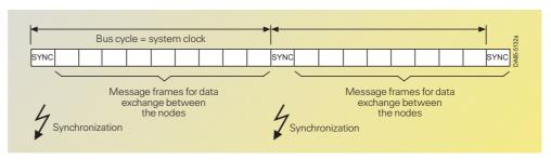
Fig. 6/76 SIMOLINK message frame communication
