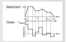
In order to select the correct drive, the speed and the load torque curves must be known.
