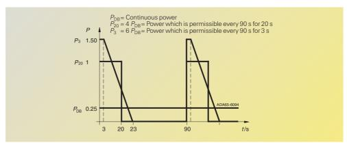
Fig. 6/53 Load diagram with **external** braking resistor
