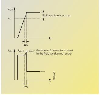
Fig. 6/5 Example of motor speed and motor torque in a time segment  $\Delta t_i$
