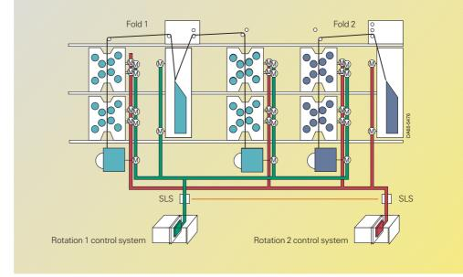
Fig. 6/79 Shaftless printing machine with SIMOLINK
