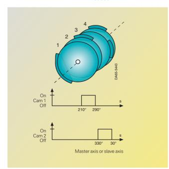
Fig. 6/85 Cam controller for MASTERDRIVES Motion Control
