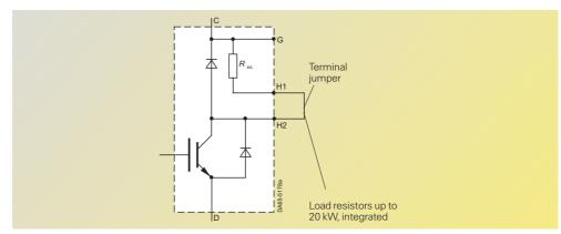
Fig. 6/50 Block diagram of a braking unit with **internal** braking resistor
