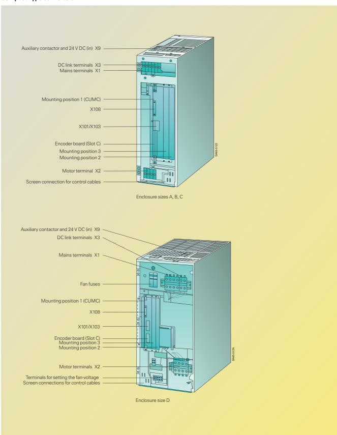
Fig. 6/38 Overview of terminals on the Compact-type converters
