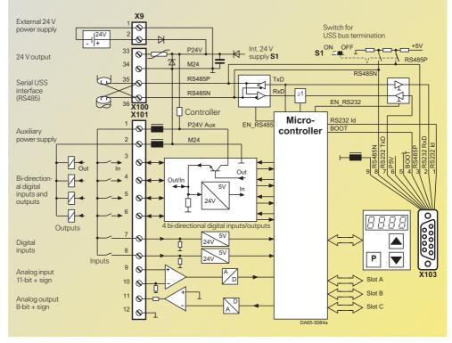
Fig. 6/32 Control terminals of Compact PLUS converters
