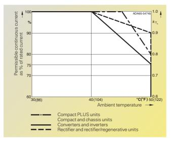
If the MASTERDRIVES units are operated at installation altitudes up to 1000 m (3282 ft) above sea level and at ambient temperatures > 40 °C (104 °F), the **current reduction factors** from Fig. 6/20 are to be applied to the rated current.
