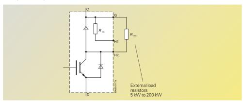
Fig. 6/52 Block diagram of a braking unit with **external** braking resistor
