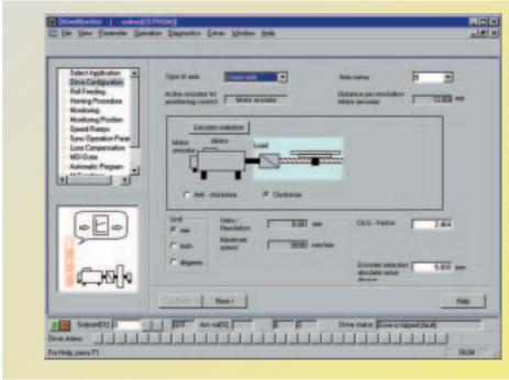
Fig. 6/89 Start-up screen form for axis configuration
