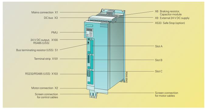
Fig. 6/30 Connection overview for Compact PLUS converters 5.5 kW (7 HP) and 7.5 kW (10 HP)
