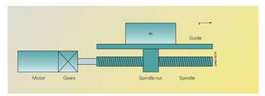
Fig. 6/1 Typical spindle drive
