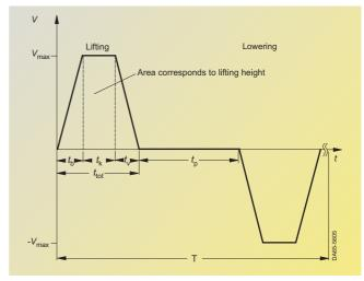
Fig. 6/13 Travel curve for lifting and lowering
