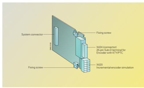
Fig. 6/61 View of the SBM2 option board
