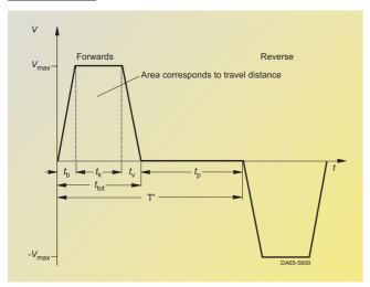
Fig. 6/8 Travel curve for forwards and reverse travel
