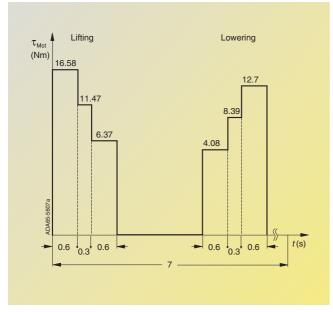
Fig. 6/15 Torque characteristic for lifting and lowering
