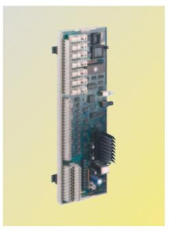
Fig. 6/70 SCI1 interface board
