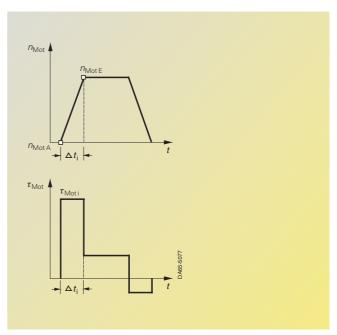
Fig. 6/4 Example of motor speed and motor torque in a time segment  $\Delta t_{\rm i}$
