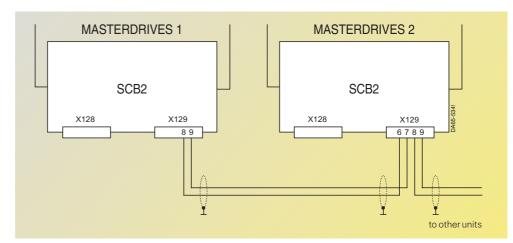
Fig. 6/67 Example of a serial peer-to-peer connection via RS485
