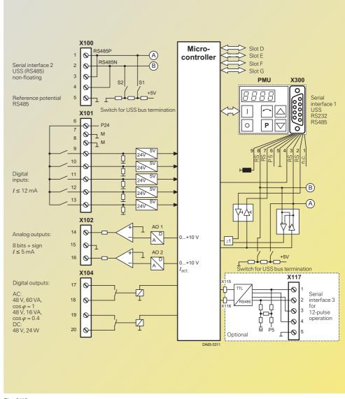
Fig. 6/42 Control terminals on the CUR control board
