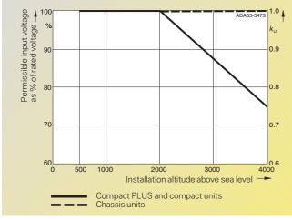
Fig. 6/22 Reduction factor  $k_{\rm V}$  for installation altitudes from 1000 m (3282 ft) to 4000 m (13126 ft) above sea level
