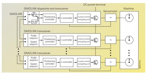
Fig. 6/78 Angular synchronism with SIMOLINK
