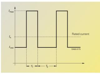
Fig. 6/18 Example of an overload curve
