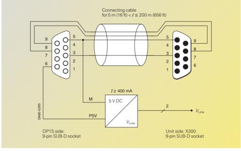
Fig. 6/98 OP1S in a point-to-point link with up to 200 m (656 ft) of cable
