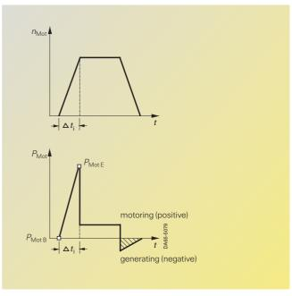
Fig. 6/6 Example of motor speed and motor output in a time segment  $\Delta t_i$
