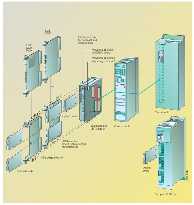
Integrating/mounting option boards in Compact PLUS, compact and chassis units.
