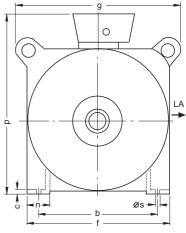
Maximum dimensions. Depending on the electrical design (terminal box type), smaller dimensions are also possible.
