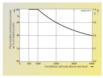
Current reduction (correction factor  $k_I$  in accordance with Fig. 6/21) is also necessary if the units are used at installation altitudes between 1000 m (3282 ft) and 4000 m (13126 ft) above sea level.
