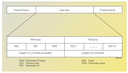
Fig. 6/74 Message frame structure with the USS protocol
