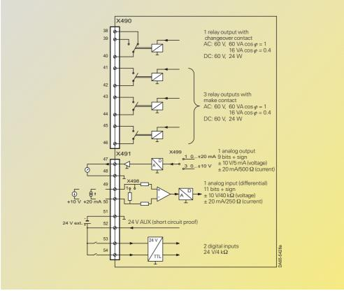
Fig. 6/65 Circuit diagram of the EB2 expansion board
