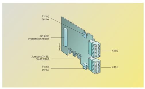
Fig. 6/62 EB1 expansion board
