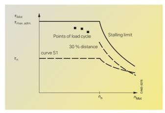
Fig. 6/3 Torque limit curves for 1PH7 motors (asynchronous servomotors)
