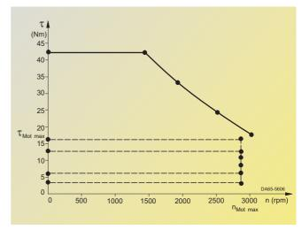
Dynamic limit curve for the 1FT6082–8AF7 with the points of the load cycle
