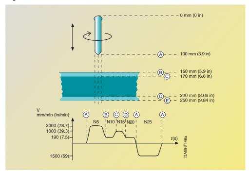
Fig. 6/90 Automatic drill function
