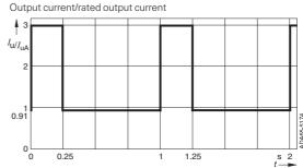
The short-time overload capacity of the Compact PLUS units is additionally limited by the  $I^2t$ -calculation (overload characteristic).
