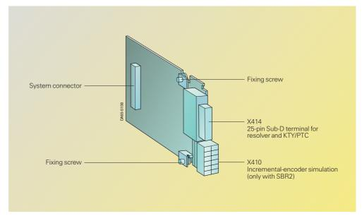
Fig. 6/59 View of the SBR option board
