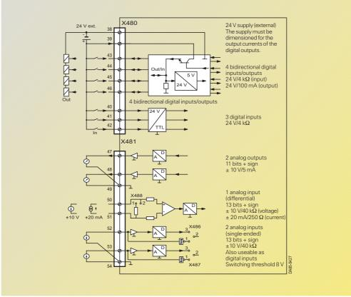
Fig. 6/63 Circuit diagram of the EB1 expansion board
