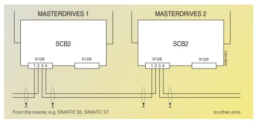
Fig. 6/69 Example of a bus connection with USS protocol via RS485.
