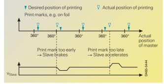
Fig. 6/93 Example of print-mark synchronization
