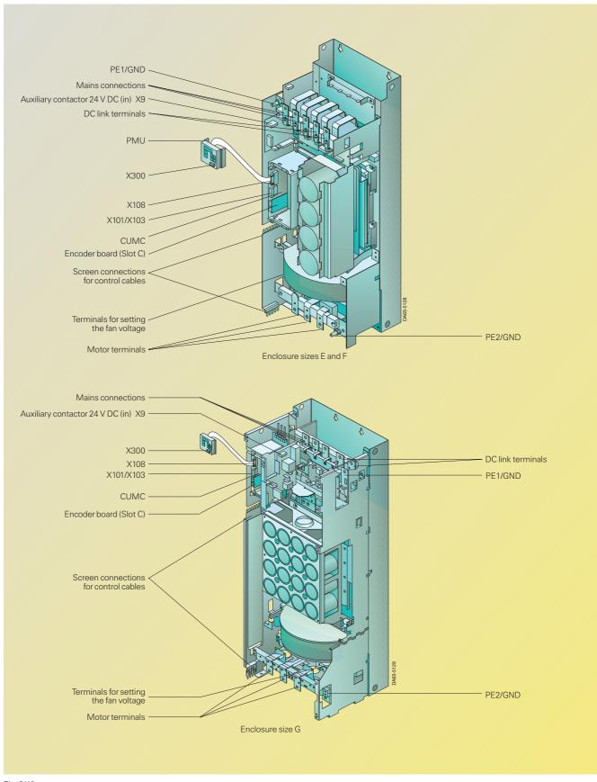
Fig. 6/40 Overview of terminals on the chassis-type converters
