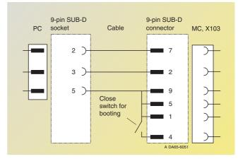
Combination cable for boot function and DriveMonitor
